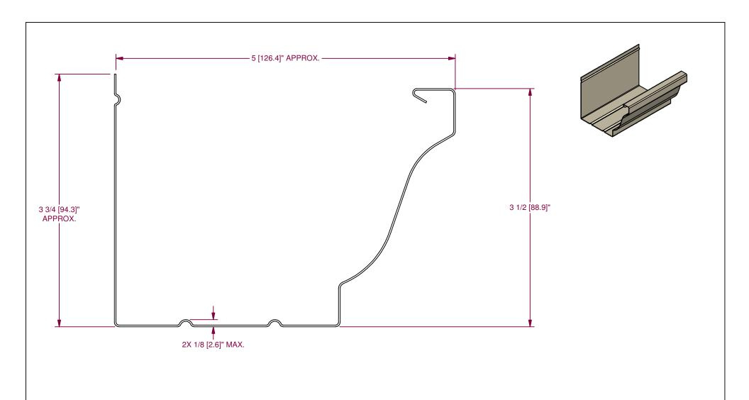
NOTE: 1. COIL WIDTH: 11 3/4" [298mm] to 11 7/8" [302mm] 2. DUAL DIMENSIONS: Inch [mm] 3. SEE MG5-SB5 FOR ADDITIONAL DIMENSIONS.
